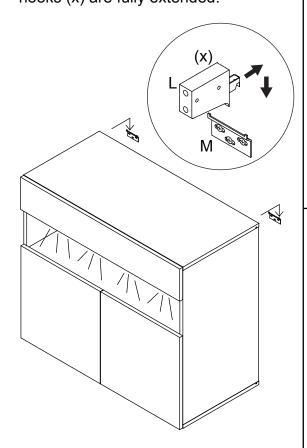
ii. With help, hang the cabinet onto the metal wall brackets by carefully aligning the end panels so they just miss the ends of the brackets. Turn upper screw(s) on either side until unit is horizontal.
